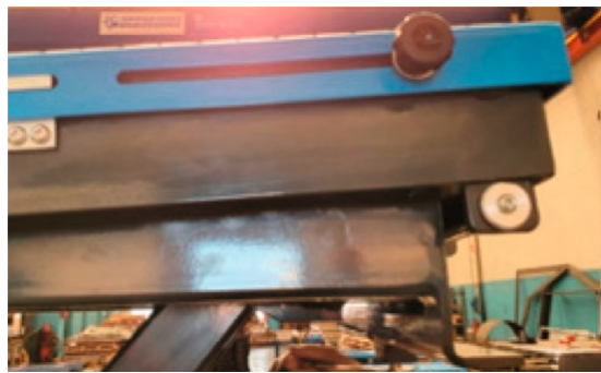
Platform tilting adjustment point and relevant pictogram
