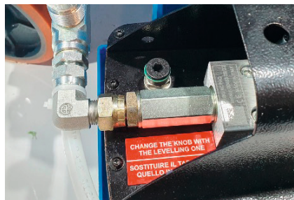
Sticker on pneumo-hydraulic pump: "replace the plug with the one supplied"
