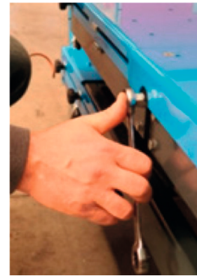
Platform movement adjustment point and relevant pictogram
